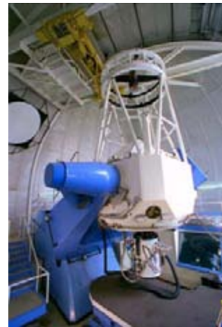
The 2.1-meter (84-inch) telescope at the Kitt Peak National Observatory, near Tucson, Arizona. The white cylinder at the bottom of the telescope is Phoenix, a new, world-class infrared spectrograph.
