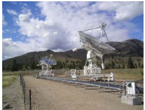
Solid center of dish shields black body radiation
