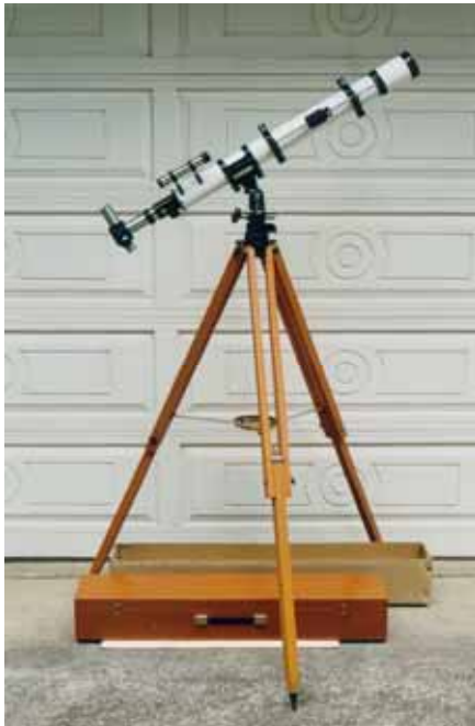
Unitron Model 114 2.4-inch altazimuth refractor telescope. An example from the 1970s of museum quality, it is easily worth $600-700.
