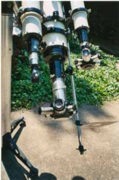
The focuser region, showing Unitron's Super-UNIHEX rotary eyepiece selector on the main scope and their Model A unit on the 2.4" guide telescope.
