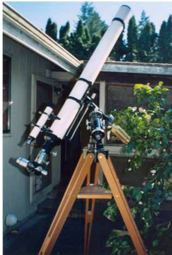
Unitron's 4" f/15 Equatorial Refractor customized by the author (circa 1958 mounting with mid-1950's optical tube, brass counterweights). Optical figuring is perfect. The large optional Super UNIH-HEX rotary eyepiece selector brings $375 alone, while the special 58mm o.d. 60mm Kellner eyepiece realizes $160-170.
