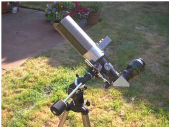
80mm f5 refractor with dew shield – yep, the eyepiece cost way more than everything else put together.
