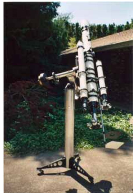
Unitron 5" f/16 refractor telescope tube assembly and auxiliary equipment remounted on a Meade Research Grade Equatorial. A superb performer, this jewel of a refractor is a favorite for double star hunting.
