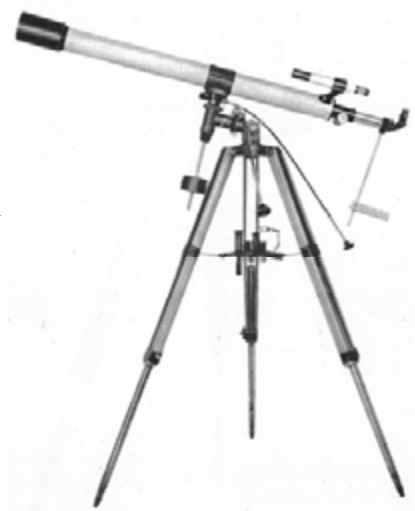
Towa Model No. 339 (D=80mm F=1200mm) as shown on the cover of the 18-page instruction manual. A common refractor, it went by a variety of different names and model numbers. The current secondary market value is $250-375.
