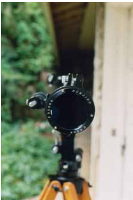
Model 114’s workhorse, an air-spaced, achromatic 2.4-inch (60mm) objective lens of 35.4-inch (900mm) focal length.
