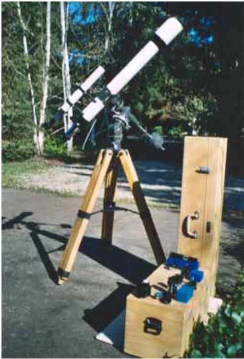
The “Arcturus” (D=76.2mm f=910mm). A complete instrument that is all-original, it even has the bill of sale dated February 23, 1961. Telescope Serial No. 070723/Objective No. 34318.
