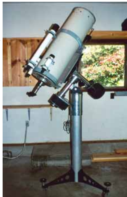
Cave Optical Co. 10" Cassegrain tube assembly remounted on a modified Meade Research Grade Equatorial for greater stability. The mirrors are from 3-B Optical Co. A work of art!
