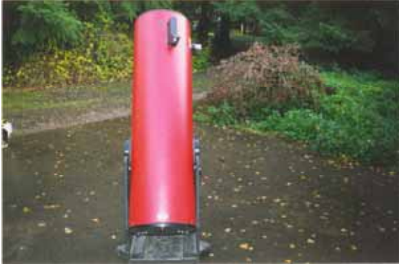
Coulter Optical® 13.1" f/4.5 Odyssey 1 "red" Dobsonian reflector telescope. This model was purchased in April 1993.
