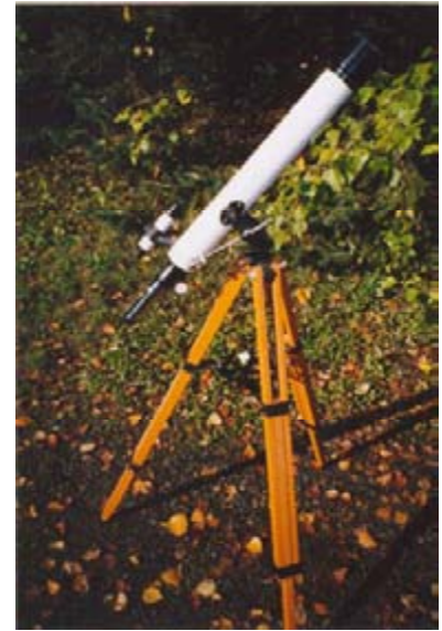
Sears Discoverer 60mm f/11.7 alt-azimuth refractor telescope, an optical winner. The current secondary market value is $50-75.
