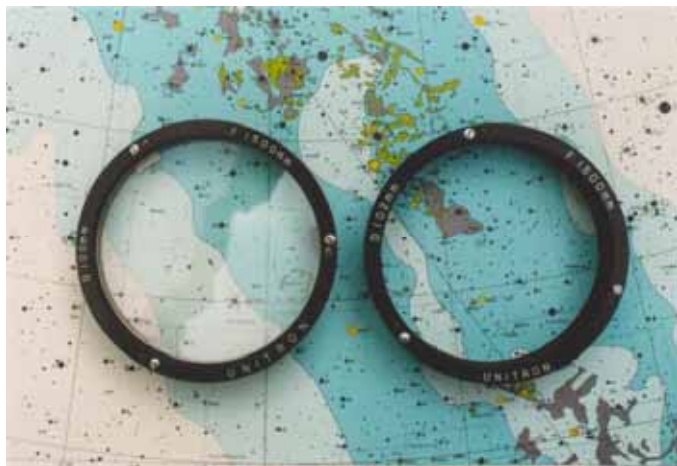
Unitron 4-inch inner objective lens cells marked D100mm and D102mm—the font spacing and size is slightly different.
