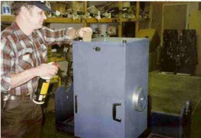
Employee putting finishing touches on a 13.1" f/4.5 Odyssey I. Photo courtesy of Mary E. Braginton.
