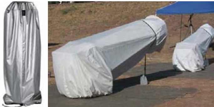
Nice scope covers, but do not leave your Dob pointing straight up during the day... the photo on the right shows a much safer orientation. Note the water jugs hanging off the front end of these
