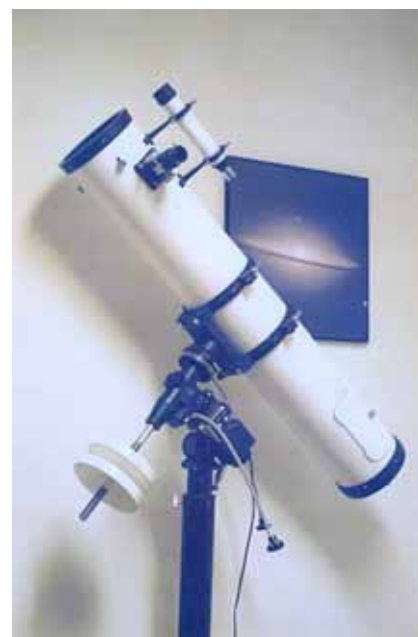
Figure 2. The author's deluxe 6-inch f/9 (1,300mm focal length) equatorial reflector telescope.
