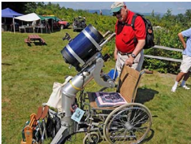
John (Jack) David Heinzmann's SCT is modified for use from a wheelchair. The eyepiece is “polar aligned” along with the RA axis, so you can point the scope anywhere without changing the observer's position.
