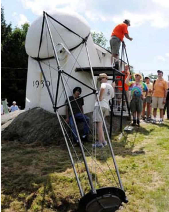
The Porter Turret Telescope. The whole truss system rotates in RA. The diagonal mirror on the edge of the dome can be rotated from inside and provides the DEC adjustment. The focused image passes through a hole in the center of the diagonal to inside the dome.
