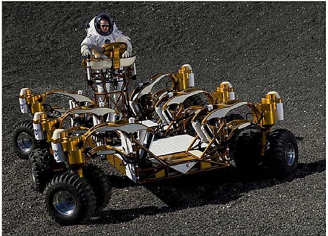
The Chariot Lunar Truck is one idea for a vehicle equal to the lunar terrain. Each of the six wheels pivot in any direction, and two turrets allow the astronauts to rotate 360°.
