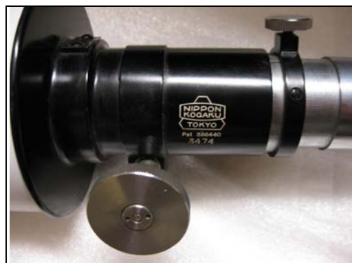
Nippon Kogaku (Nikon) placed an especially nice rack-and-pinion focuser on its 65mm refractor telescopes (above). Right: A rotating unit provides the necessary focusing on this 3-inch f/12 instrument from Lafayette Radio.
