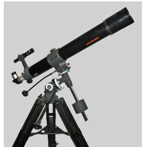
Celestron's Firstscope 80EQ was used for several of the needed deep-sky observations.
