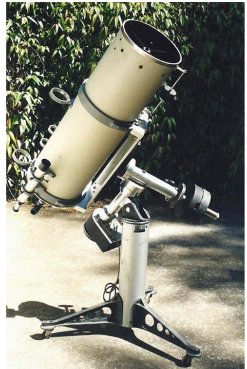
A 10-inch Cave Astrola Cassegrainian-style reflector sits atop a massive Meade Research Grade equatorial mounting in this deep-sky observer's setup.
