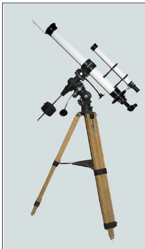
Nippon Kogaku (Nikon) placed an especially nice rack-and-pinion focuser on its 65mm refractor telescopes (above). Right: A rotating unit provides the necessary focusing on this 3-inch f/12 instrument from Lafayette Radio.
