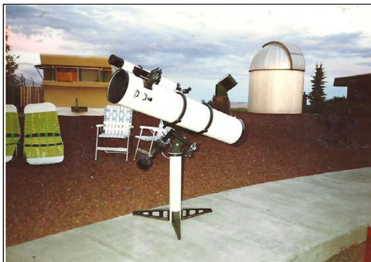
Patterned after the venerable 1960's Optical Craftmen 'Discoverer' series of 8-inch telescopes, this customized reflector awaits nightfall at Washington's Golden-dale Observatory.
