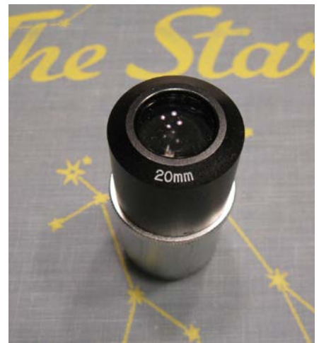
These lightweight 20mm Erfles were once advertised by Meade. (Cave listed them in its catalogs as "Orthostars.") The popular series also included 7, 12.4 and 15.5mm focal lengths.
