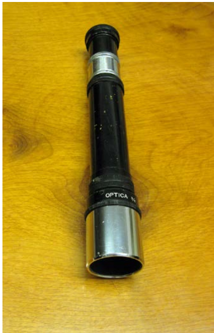
Top: Turret holders are designed to switch between different slots at the observer's touch. The selector on the Sears 90mm refractor telescope holds up to six color-coded 0.965-inch oculars. Above: Optica b/c's 8-21mm zoom lens replaces two or more expensive eyepieces. Right: A private collection of 1960's University Optics orthoscopic eyepieces with their original boxes.
