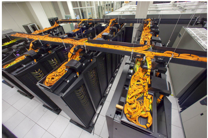
The Carver IBM iDataPlex supercomputer at NERSC at Lawrence Berkeley National Laboratory does much of the real-time analysis of images for the PTF, comparing digital images taken with the 48-inch Samuel Oschin telescope on Mount Palomar with reference images to identify supernovae. It found SN 2011fe.
